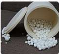
Corundum tank and zirconia balls
