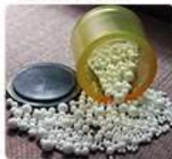
Polyurethane (pu) tank and zirconia balls
