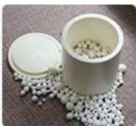
zirconia tank and balls
