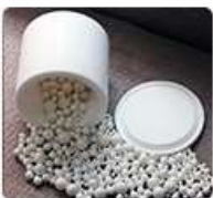
Ptf e tank and zirconia balls
