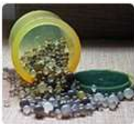
Polyurethane (pu) tank and agate balls
