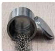
cemented carbide tank and balls
