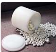
Nylon tank and zirconia balls
